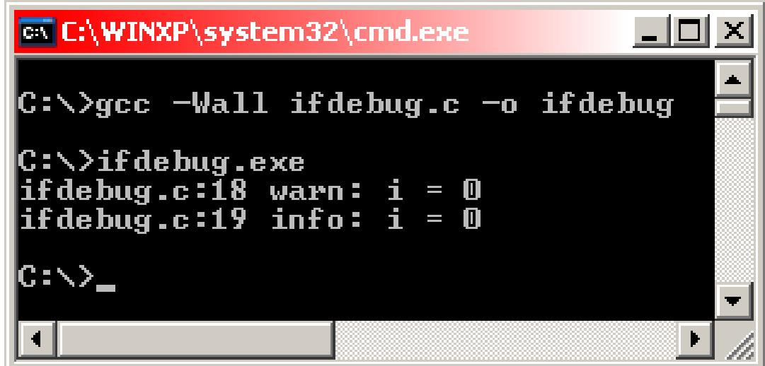
The screenshot shows a Windows command prompt window titled 'cmd C:\WINXP\system32\cmd.exe'. The command entered is 'C:\>gcc -Wall ifdebug.c -o ifdebug'. The output shows two lines of debug information: 'ifdebug.c:18 warn: i = 0' and 'ifdebug.c:19 info: i = 0'. The window has standard XP-style borders and a scroll bar.
